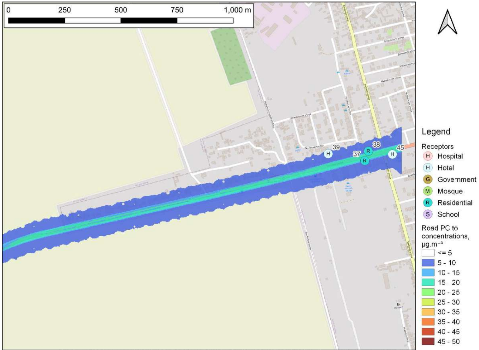
Figure 1-24: Road PC to maximum 24-hour mean NO 2 concentrations with project, 2027: Karakol, \mu\text{g}\cdot\text{m}^{-3}
