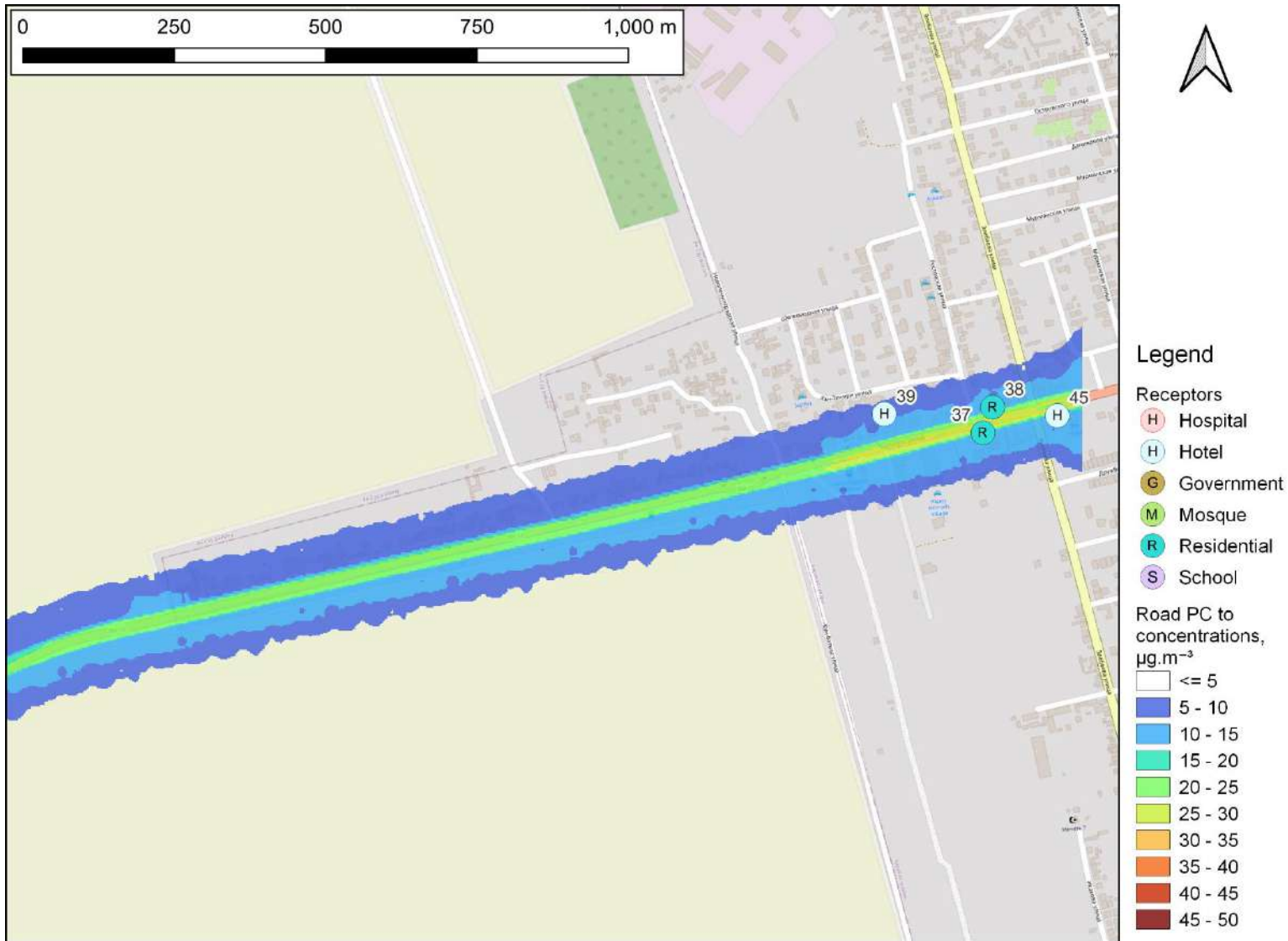
Figure 2-24: Road PC to maximum 24-hour mean NO 2 concentrations with project, 2047: Karakol, \mu\text{g}\cdot\text{m}^{-3}
