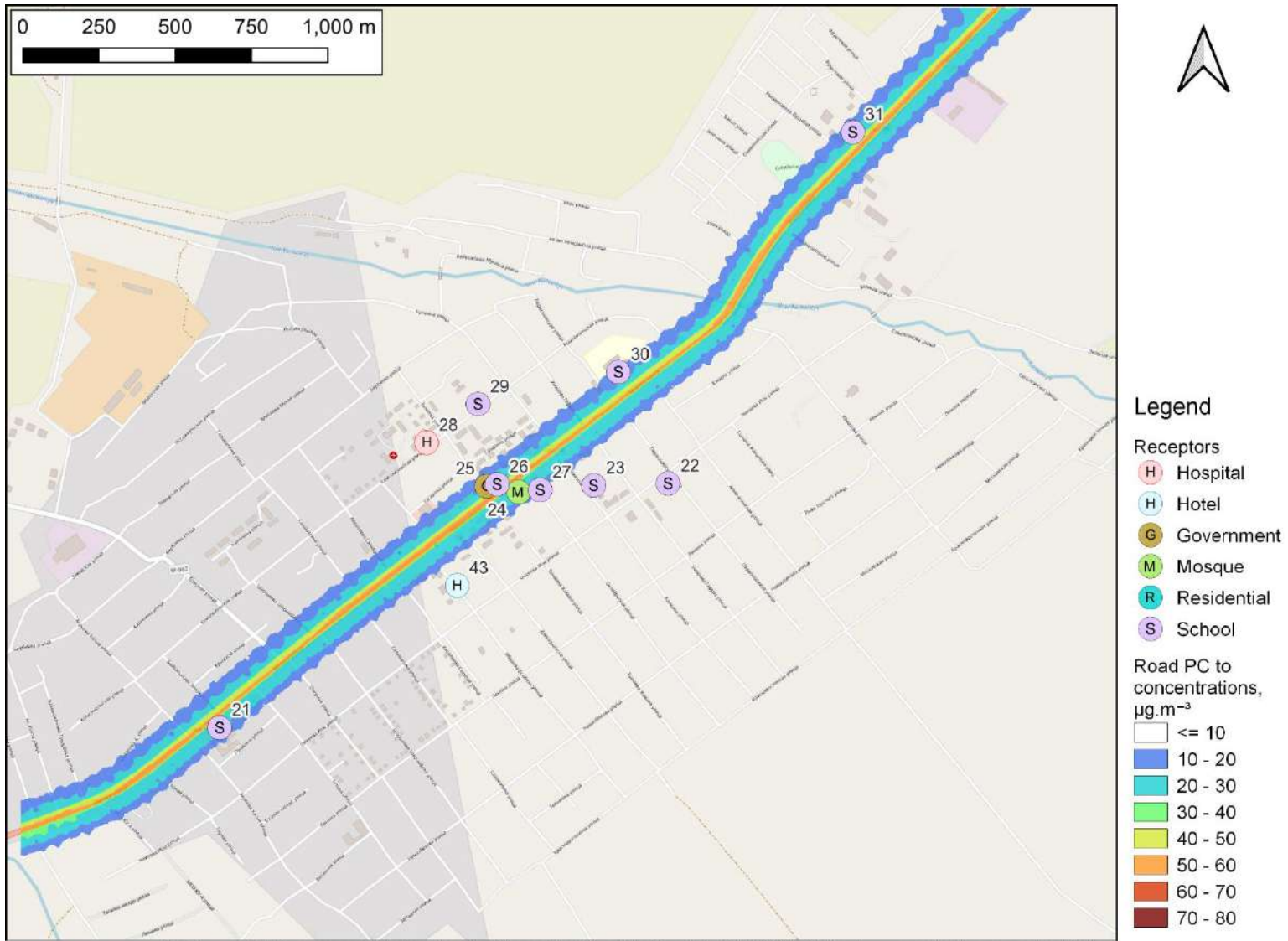
Figure 2-5: Road PC to 99 th percentile of 24-hour mean PM 10 concentrations with project, 2047: Kyzyl Suu, \mu\text{g}\cdot\text{m}^{-3}
