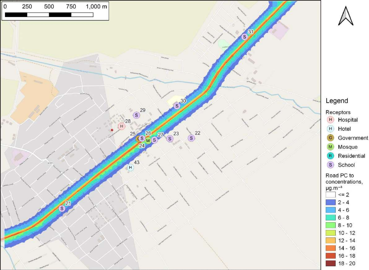
Figure 1-14: Road PC to 99 th percentile of 24-hour mean PM 2.5 concentrations with project, 2027: Kyzyl Suu, \mu\text{g}\cdot\text{m}^{-3}
