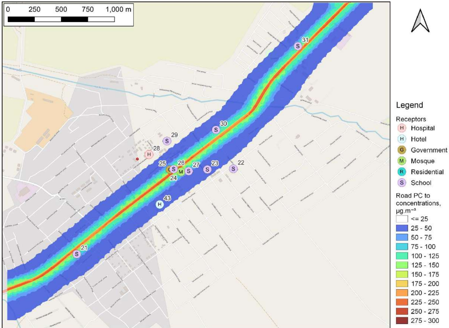
Figure 2-8: Road PC to maximum of 1-hour mean PM 10 concentrations with project, 2047: Kyzyl Suu, \mu\text{g}\cdot\text{m}^{-3}
