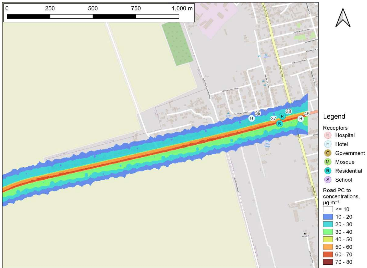
Figure 1-6: Road PC to 99 th percentile of 24-hour mean PM 10 concentrations with project, 2027: Karakol, \mu\text{g}\cdot\text{m}^{-3}
