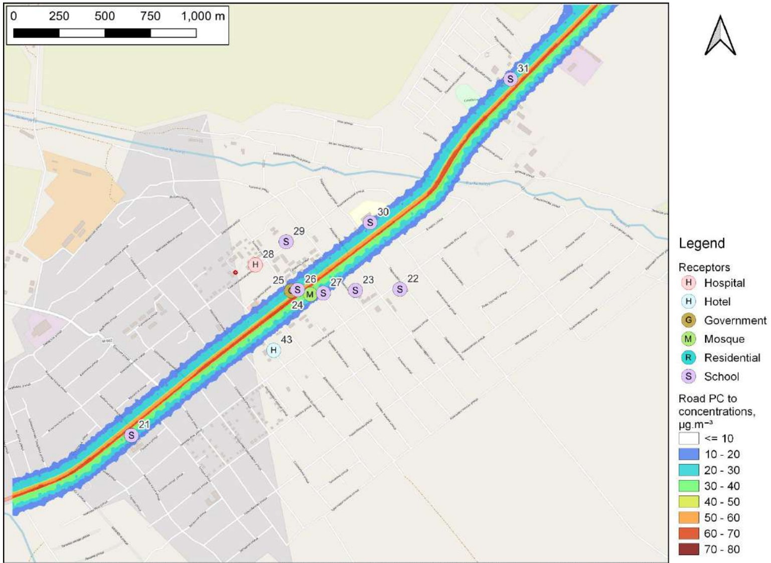
Figure 1-5: Road PC to 99 th percentile of 24-hour mean PM 10 concentrations with project, 2027: Kyzyl Suu, \mu\text{g}\cdot\text{m}^{-3}
