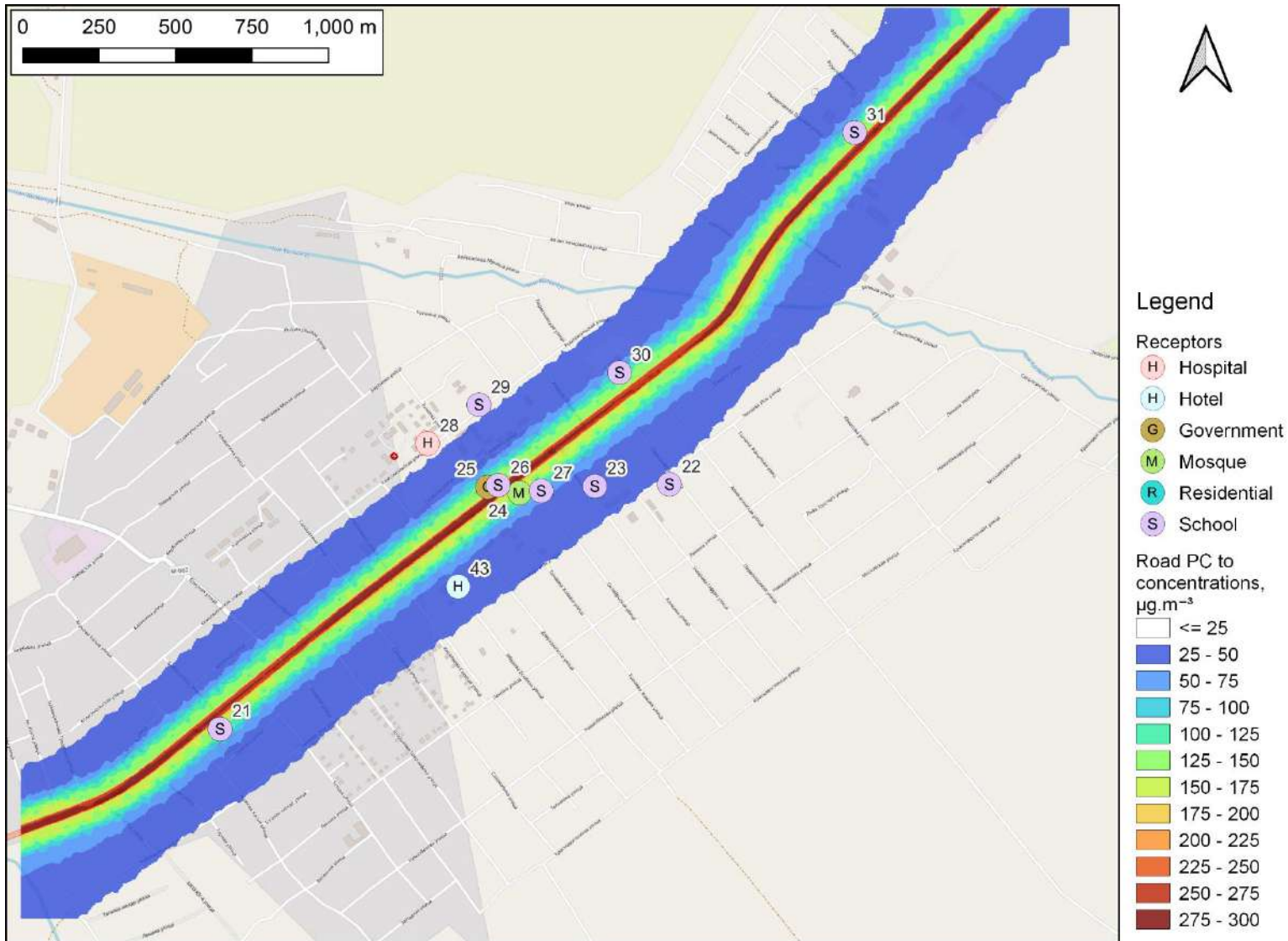
Figure 1-8: Road PC to maximum of 1-hour mean PM 10 concentrations with project, 2027: Kyzyl Suu, \mu\text{g}\cdot\text{m}^{-3}
