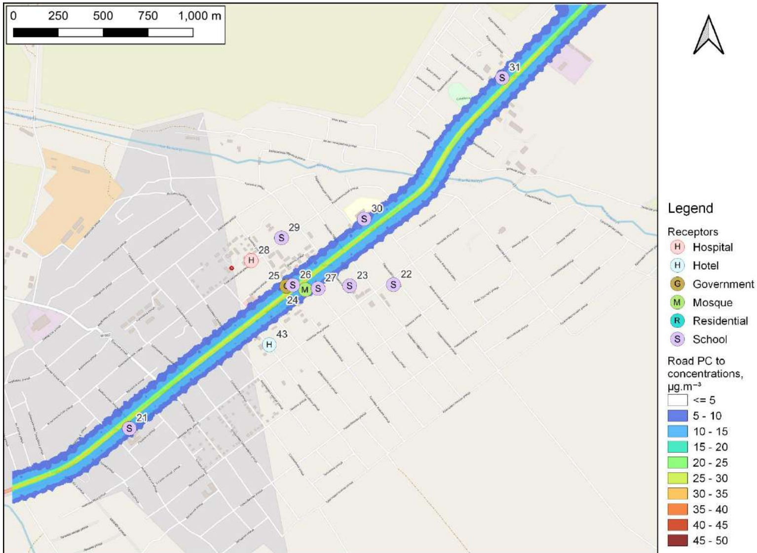
Figure 2-23: Road PC to maximum 24-hour mean NO 2 concentrations with project, 2047: Kyzyl Suu, \mu\text{g}\cdot\text{m}^{-3}
