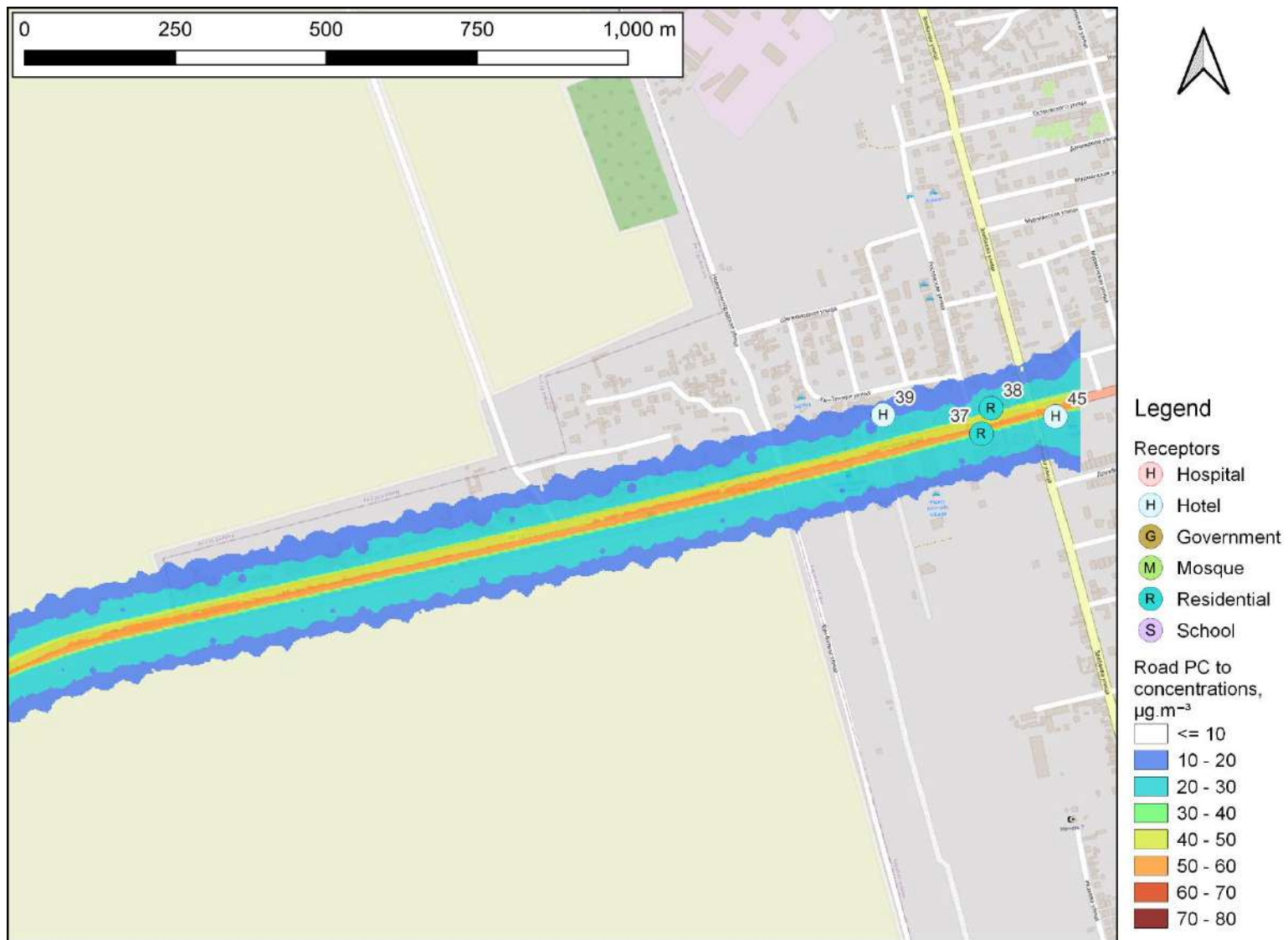
Figure 2-6: Road PC to 99 th percentile of 24-hour mean PM 10 concentrations with project, 2047: Karakol, \mu\text{g}\cdot\text{m}^{-3}
