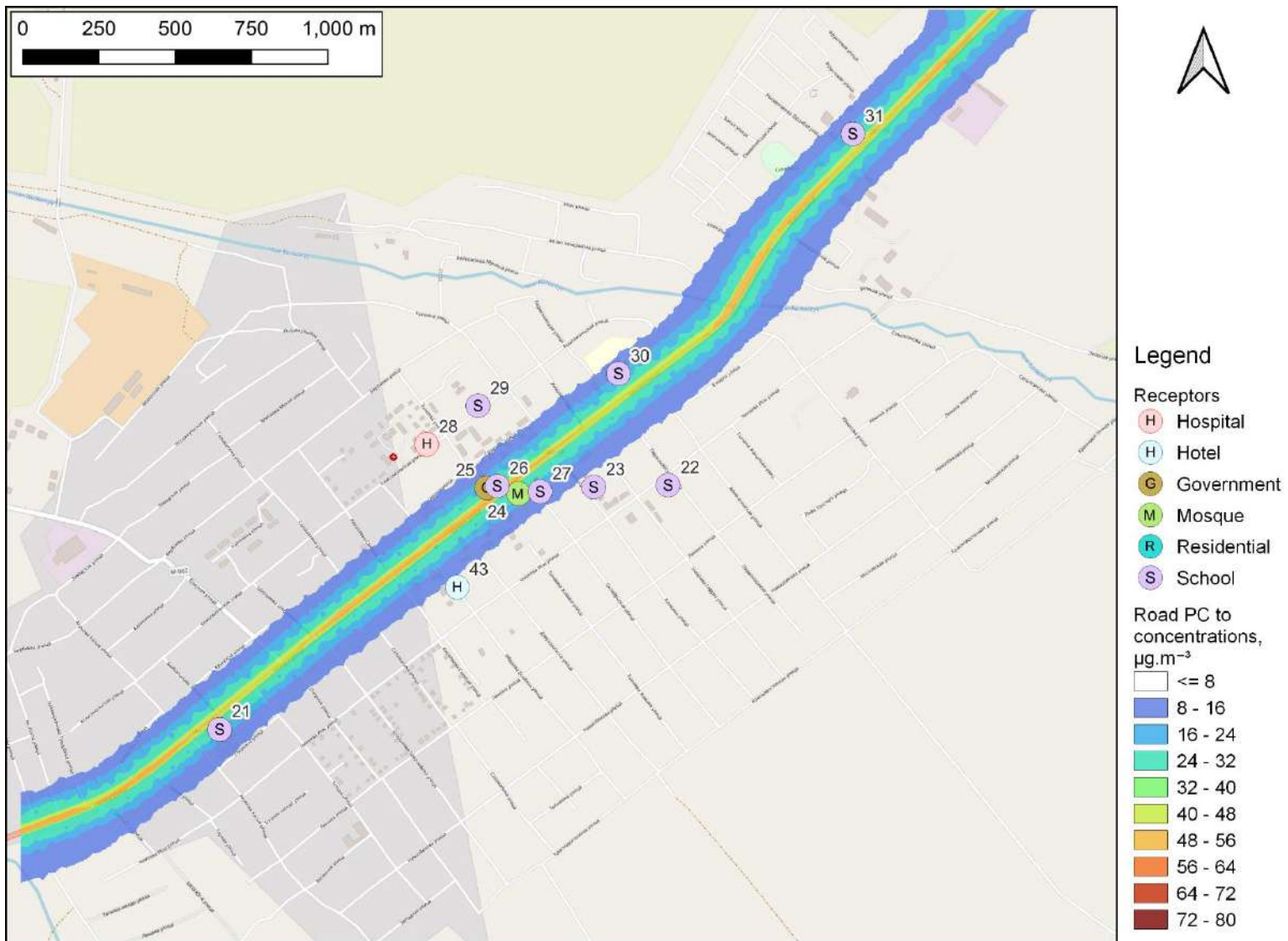
Figure 2-17: Road PC to maximum of 1-hour mean PM 2.5 concentrations with project, 2047: Kyzyl Suu, \mu\text{g}\cdot\text{m}^{-3}
